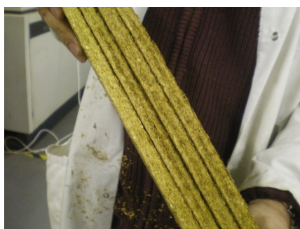
Figure 50. Delamination in the midline of a milk hardener board which had blown when the press opened. This is sometimes only visible once the panel is cross cut for quality checks, as shown.
