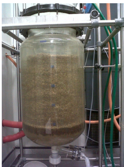
Figure 17. 50 litre dewaxing of wheat straw. At the start of the reaction the straw bulk floats above the ethanol with only partial mixing (shown), but as dewaxing proceeds the straw becomes better wetted with ethanol.
