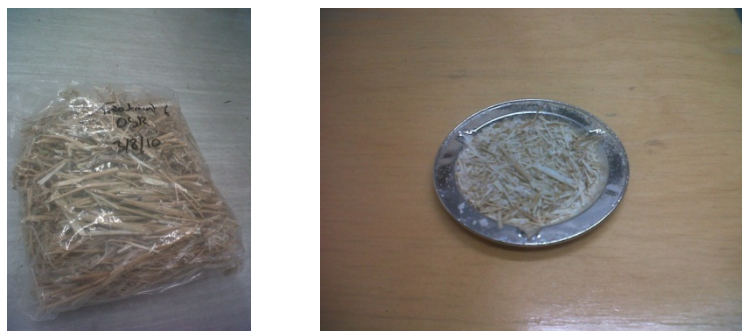
Figure 42 a. Oilseed rape stems in a range of different diameters, as supplied for analysis. b. Oilseed rape particles after hammer milling.
